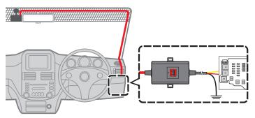
Connect the Smart Box II to the recorder and confirm it is working properly by the LED indicator that glows in red. Then you can arrange the cable and complete the installation.
