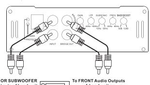
To REAR OR SUBWOOFER Audio Outputs of head unit or signal processor
